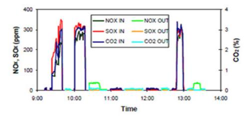
Typical CO<sub>2</sub> composition of propane combustion flue gases, before and after entering the full scale PBR (25,000 liter) microalgal photobioreactor, are shown in Figure 12. On average, the mass calculations indicate that the microalgal culture was able to capture about 45% of the available CO<sub>2</sub> when the culture was maintained at pH 7.5.
